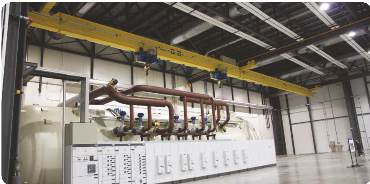
MULTIPOINT SINGLE GIRDER UNDERSLUNG CRANE. CAPACITY UP TO 20+20t.
